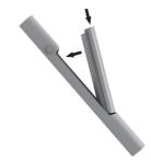
4. Now push the top part of the battery into the frame, until you hear the battery lock into position.
